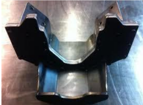
Sample Gas tank protector: Note ALL components must be 4" from sheet metal.
